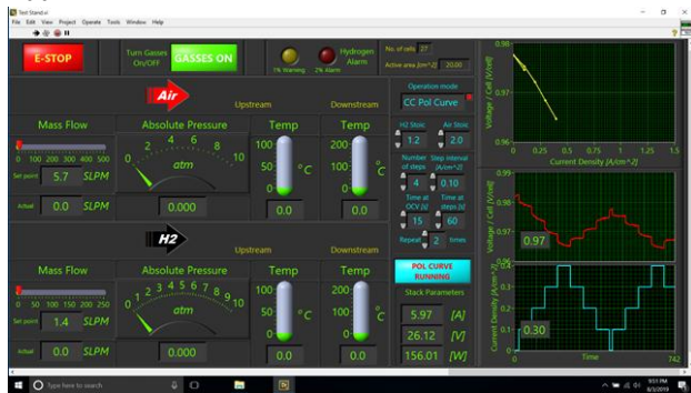
Figure 7. GUI controller for the fuel cell test stand.
