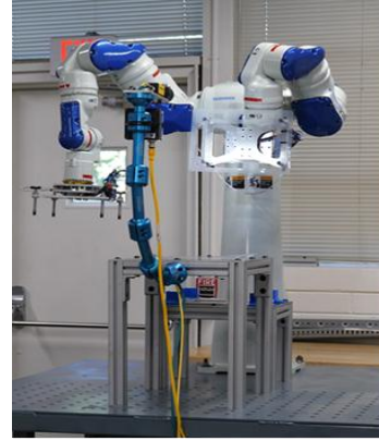
Figure 1. Yaskawa Motoman SDA5F dual arm robot with COGNEX In-Sight 8000 vision system used for automated sorting, reorientation and stacking fuel cell components in preparation for a subsequent robotic assembly process.
