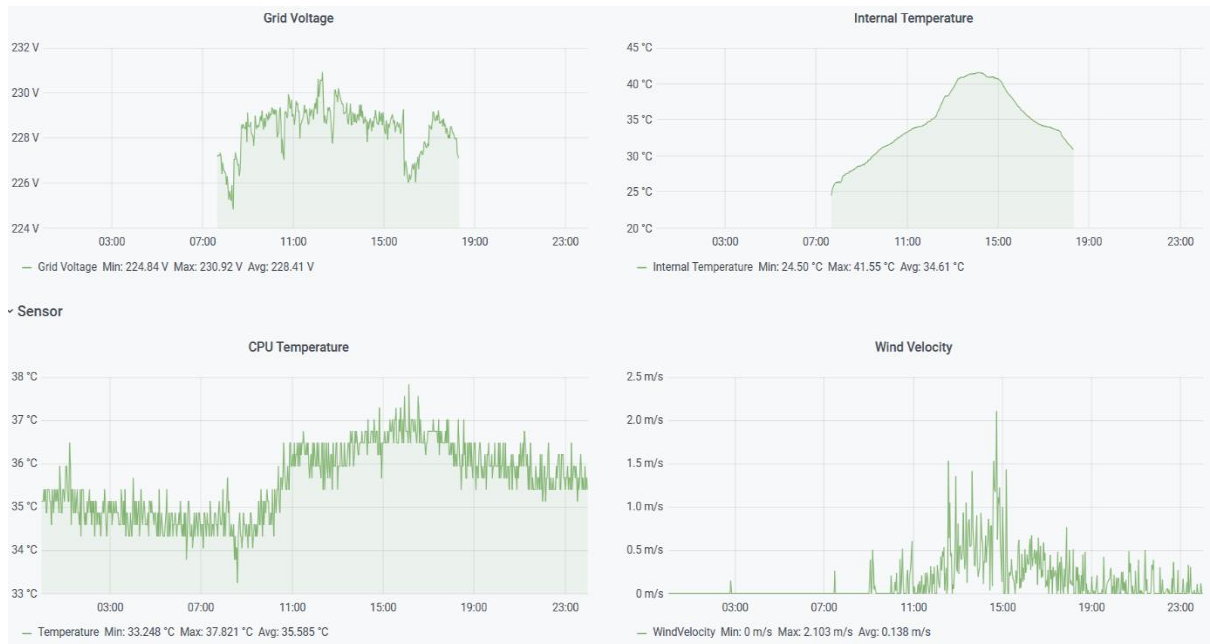
Fig. 15. Grid voltage, inverter temperature, CPU temperature and wind velocity values for 15 October 2020.
