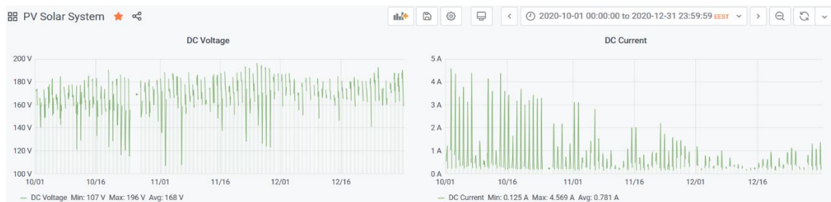
Fig. 7. DC voltage and DC current values from 1 October, 2020 to 31 December, 2020.
