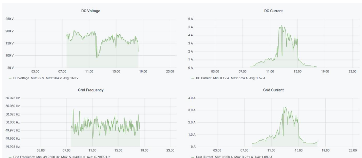
Fig. 14. DC voltage, DC current, grid frequency and grid current values for 15 October 2020.
