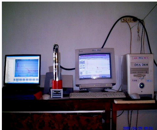
Figure 8. Gamma spectrometry with Multi-channel analyzer system
