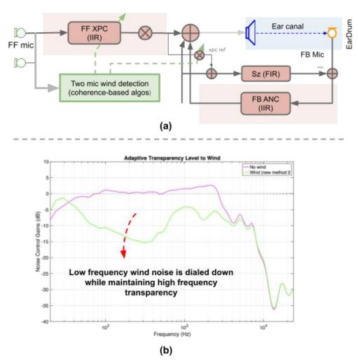
Fig. 4: Gain of an FIR filter is adjusted based on detected wind noise
