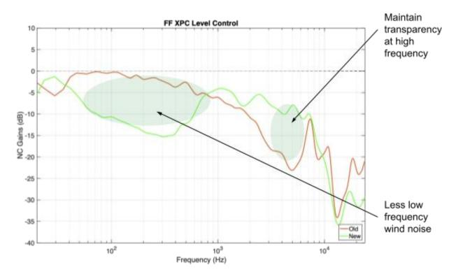
Fig. 6: Acoustic performance comparison
