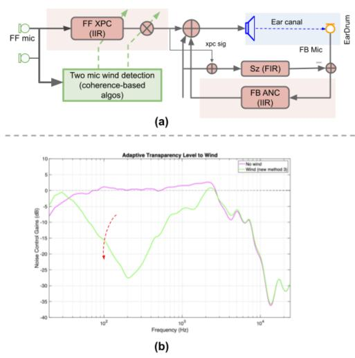
Fig. 5: Gain of the XPC filter is adjusted based on the detected wind noise
