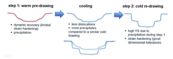
With this control of precipitation, this process allows for an improved formability and a high final strength, with no post-form heat treatment needed. This also can give rise to higher strength with a low temperature paint bake cycle.
