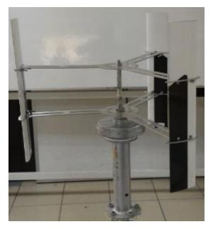
**Figure 2.2:** Lab Scale Model for the VAWT 2.2 *Experimental Set-up and Procedures*
