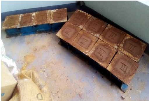
Figure 4: Cubes in the moulds
