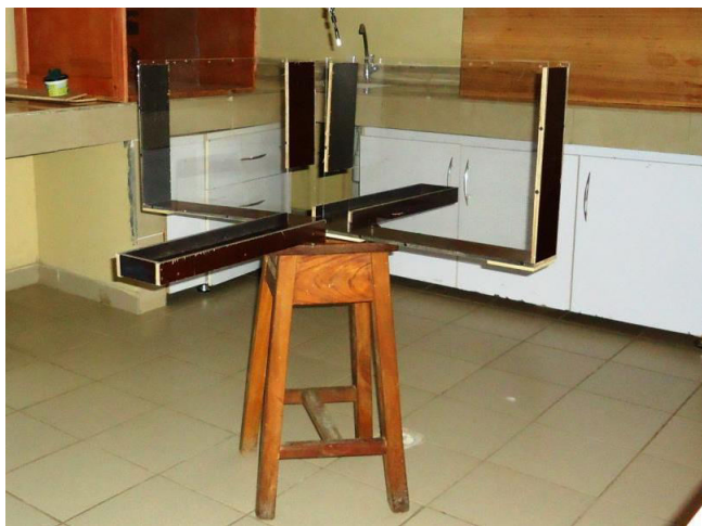
Fig. 1: The Elevated Plus Maze Box
