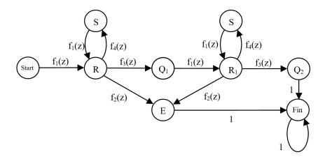
Fig.1. The graph modeling for the request service reservation productivity of a radio channel
