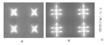
**Fig.3.** Orientation of the diffuser "Prism" optical elements with respect to the LED series: a) at the angle of 45 °; 6) in parallel; B) - the location of LEDs on the series shown in Figure
