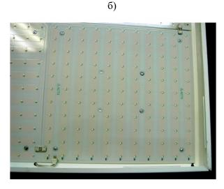
Fig.4. The location of 121 LEDs on <sup>1</sup>/<sub>4</sub> of the fixture area
