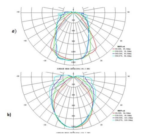
**Fig.7.** LIC of the luminary LPO46 with LED modules: a - without additional diffuser; b - with an additional opal diffuser
