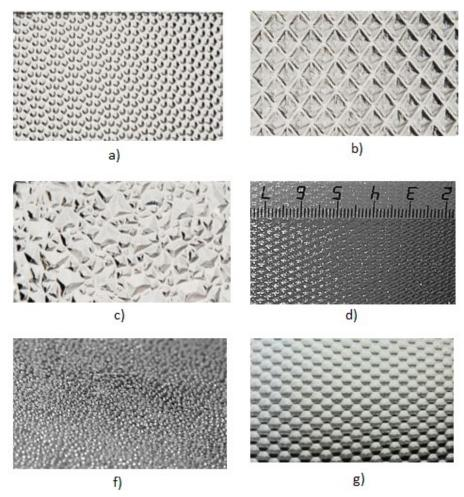
Fig.1. Diffusers for luminaires "Pin spot" (a), "Prism" (b), "Crushed ice" (c), "Microprism" (d), "Manka" (e), "Honeycomb" (f)
