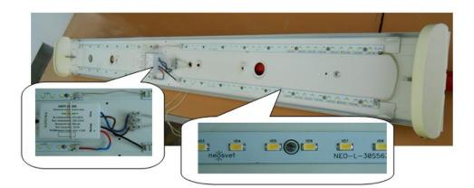
Fig.5. The location of LED modules and direct current source on the basis of the lamp LPO46
