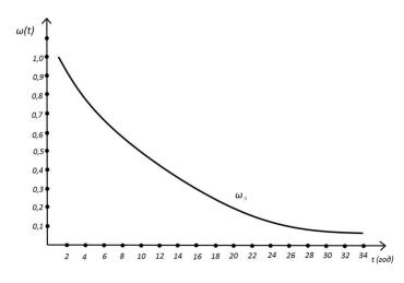
Fig.3. Dependence of quality parameters on time - welding joint  $(\omega_3)$
