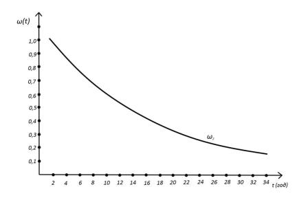
**Fig.2.** Dependence of quality parameters on time - shop weld  $(\omega_2)$
