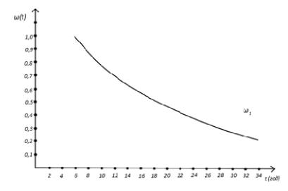
**Fig.1.** Dependence of quality parameters on time –base metal of pipes  $(\omega_1)$
