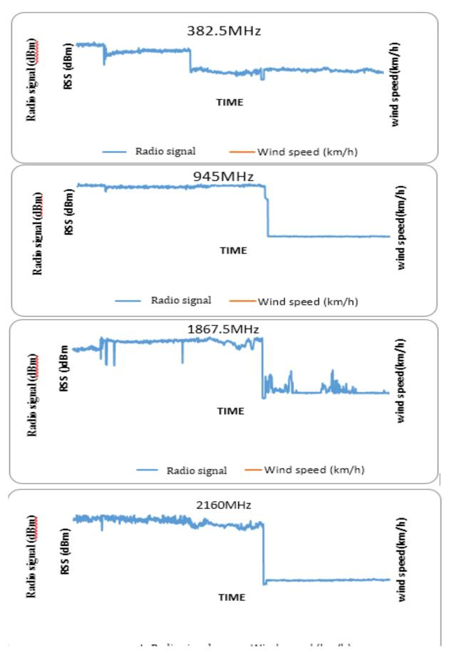
Fig.2. Graph of radio signal, wind speed versus time for 4 prominent peaks at February 2016
