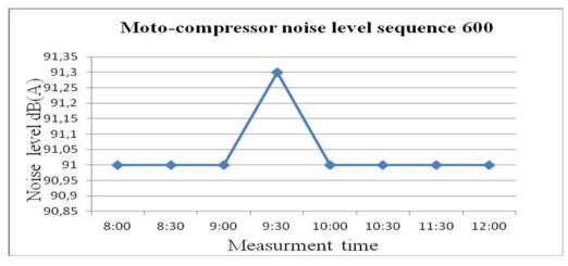
Fig.7. Noise level recorded in sequence 600
