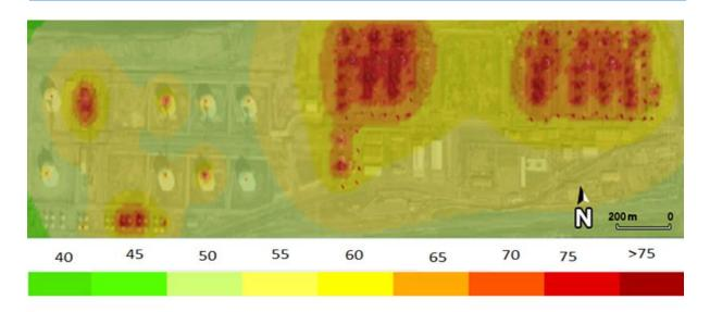
Fig.10.General noise mapping of the GP1Z plant
