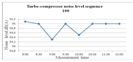
Fig.5. Noise level recorded in sequence 100
