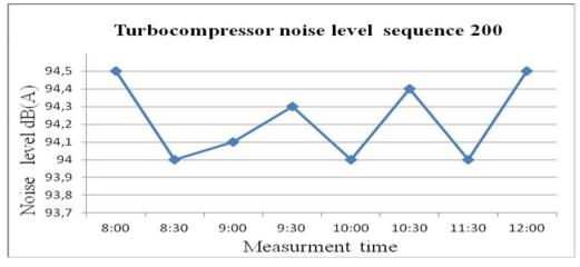
Fig.6. Noise level recorded in sequence 200
