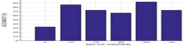
Fig.4. No of hidden unit vs testing accuracy for MLP1 (without LLE)
