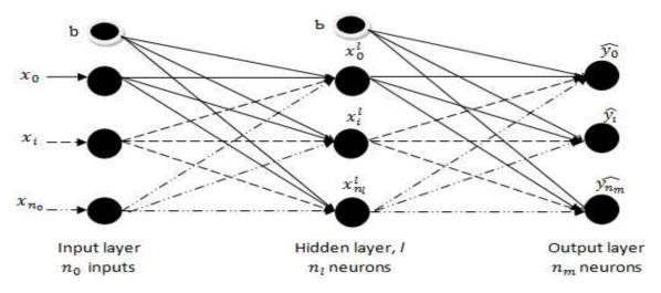
**Fig.1.** A multilayer feed forward neural network [6]
