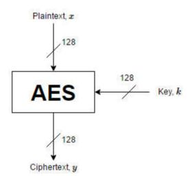
Fig.1. The general structure of AES
