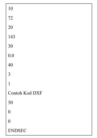
Fig.2. DXF code for text entity
