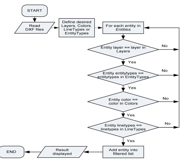
Fig.3. Flow chart of entity filtering technique
