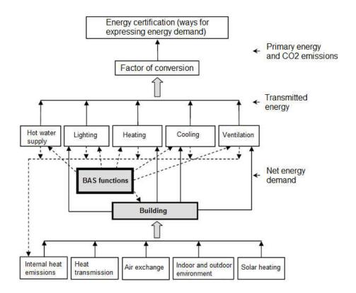
Fig.1.5. Calculation stages to determine BAS and USMT impact on the energy performance level of a building
