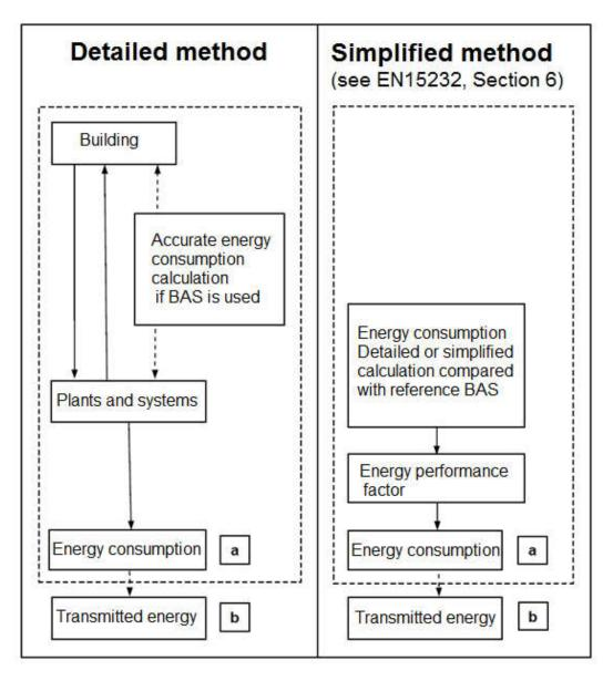
**Fig.1.6.** Detailed and simplified calculation of BAS functions impact on energy performance of a building according to EN15232: 2012
