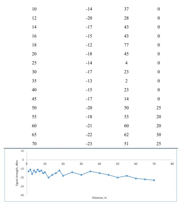
Fig.9. Signal strength versus distance of antenna performance for 2.4GHz
