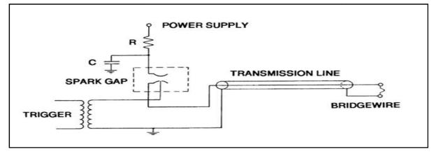
Fig.2. Basic circuitry of exploding bridge wire [11]
