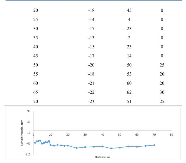
Fig.8. Signal strength versus distance of antenna performance for 5GHz
