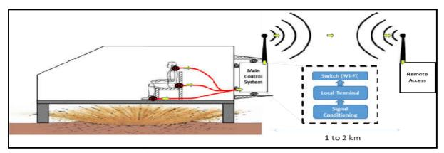
Fig.5. Previous proposed blast experiment [10]
