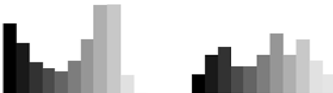
Fig.4. Greyscale intensities histograms for image in Fig. 1 with some pixels' number reduced in certain bins resulted from quantization process
