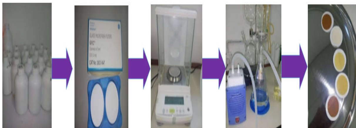
Fig.2. a) Sample water b) Membrane filter c) Electronic weighing d) Filtration apparatus
