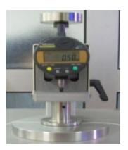
Fig.3. Thickness gauge
