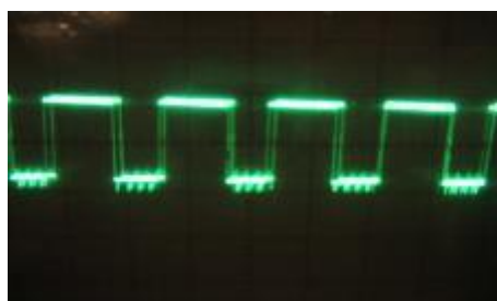
Fig. 16. Diagram voltage – time .Output of PVDF in speed 300RPM
