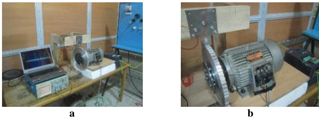
Fig. 7. (a) Electric motor, three-phase electricity is fed and the flywheel on the motor shaft is fixed thorns by means of thorns, bolts and spur. Piezoelectric output before entering the oscilloscope, will enter orbit and voltage versus time graph is visible. (b) The base engine is fixed on board the wooden by bolts and in ways that minimize vibrations have been balance.
