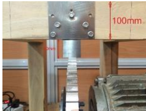
Fig. 10. How to deal flywheel teeth with end of the beam
