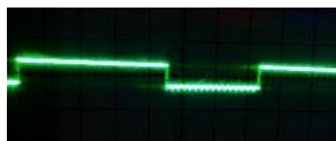
Fig. 18. Diagram voltage – time. Output of PVDF in speed 200RPM
