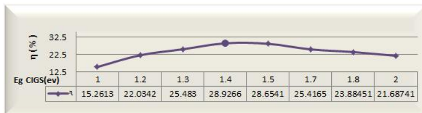
Fig.11. Performance of CIGS cell as a function of the band gap energy of CIGS absorber layer
