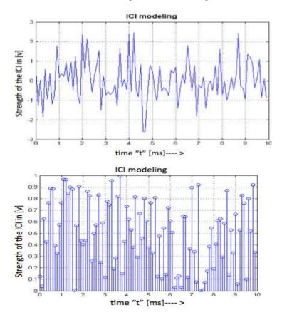
Figure 1. Shot Noise model: SN model in continuous signal (top), and SN model in discrete signal (bottom)
