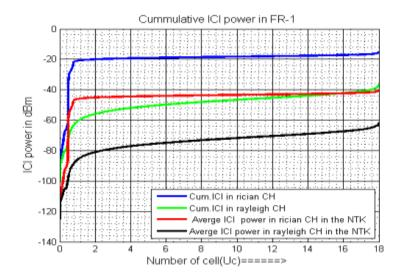
Figure 8. Cumulative and average effect of ICI power under various channel environment for FR-1 network
