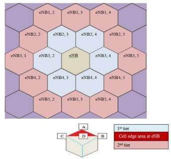
Figure 2. System network model
