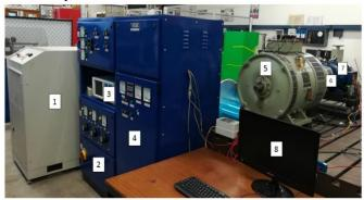
Fig. 3. The 22 kW Experimental Test Rig: 1. Programmable power supply MX 30, 2. Power supply panel, 3. Yokogowa WT1800 Power Analyzer, 4. 4-Quadrant DC Drive Load Assembly, 5. 15kW DC Machine, 6. In-line torque transducer-Magtrol TM 300, 7. Induction motor, 8. Data acquisition pc.
