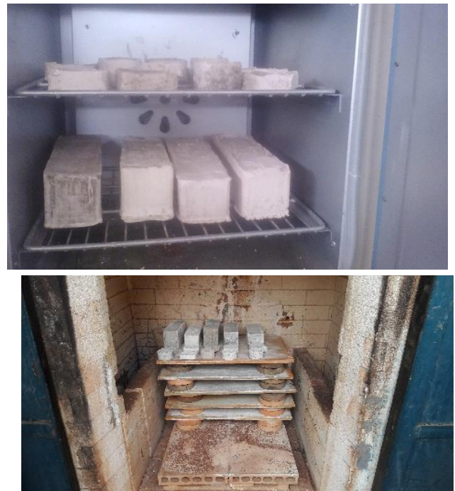
Figure 1: A picture showing the different sizes of the insulating refractory bricks (a) while still inside the oven at 110^\circ\text{C} and (b) after sintering in the furnace.
