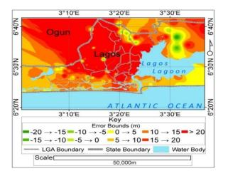
Figure 11: Surface model of  $\Delta H_{ASTER-GPS}$  showing error bounds.
