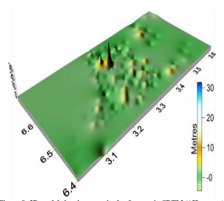
Figure 8: 3D model showing magnitude of errors in SRTM (ΔH<sub>SRTM-GPS</sub>).
