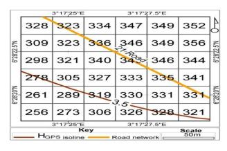
Figure 5: ASTER pixel values compared with a H<sub>GPS</sub> contour at Festac Town, Lagos.
