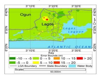
Figure 10: Surface model of  $\Delta H_{SRTM-GPS}$  showing error bounds.
