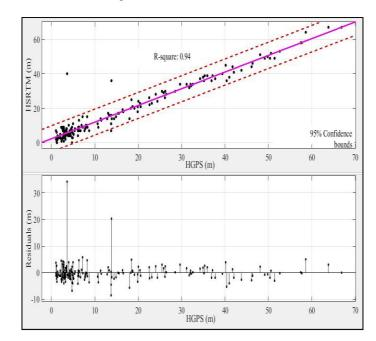
Figure 2: Visual comparison of  $H_{SRTM}$  vs.  $H_{GPS}$ : expression of 95% confidence zone (above) and residuals plot (below).
