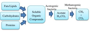
Figure 1: Schematic biochemical process stages of anaerobic digestion (Source: Achinas and Euverink, 2016)
