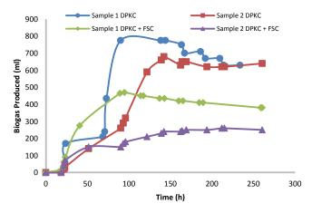
Figure 7: Cumulative biogas production with time.
