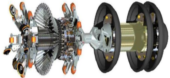
Figure 6: Geometry inspection tool (Baker Hughes, 2015).
