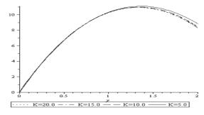
Figure 5: Effects of Permeability parameter on velocity profile
