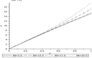
Figure 10: Effects of Magnetic number on velocity profile for (Gr < 0)
