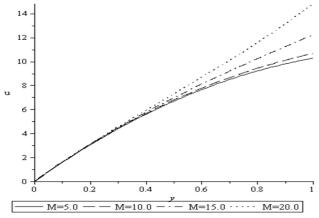
Figure 4: Effects of Magnetic number on the velocity profile
