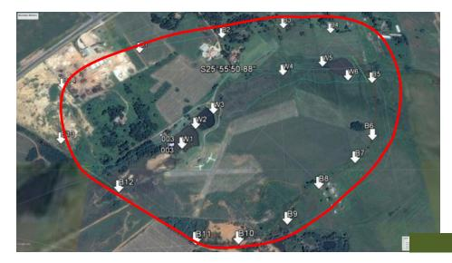
Figure 3. Ground control markers (arrows) positioned at the boundaries of the UAV survey area/study area (red line) including next to the watercourse at different elevations
