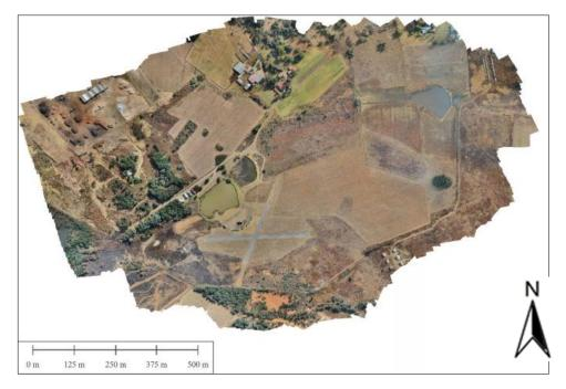
Figure 8. A 10cm ground pixel resolution orthophoto derived from the point cloud for the 100ha study area
