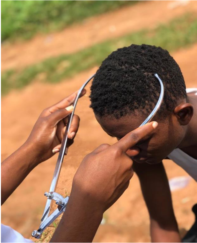
Figure 1: Measurement of the cephalic breadth using a spreading caliper.
