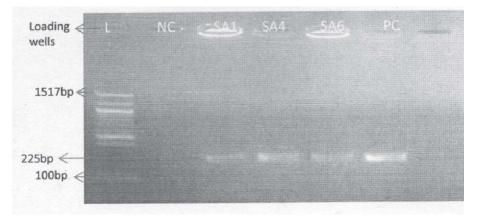
Plate 3: Molecular identification of *Staphylococcus aureus* using polymerase chain reaction technique. Isolates L: 100-1517bp DNA ladder; NC: Negative control; PC: positive *Staphylococcus aureus* control strain with American type culture collection number **29212**.
