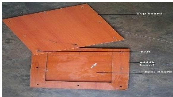
Figure 1: Mould box construction
