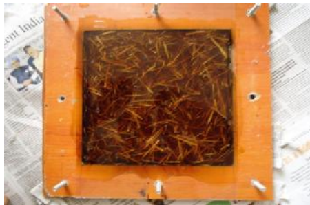
Fabrication of composite step1 Figure10: Fabrication of composite step 2
