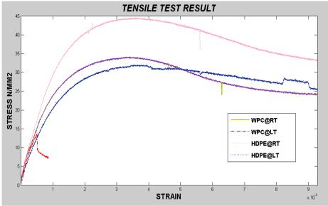
Figure 1: Stress Strain relationship for the entire tensile test.
