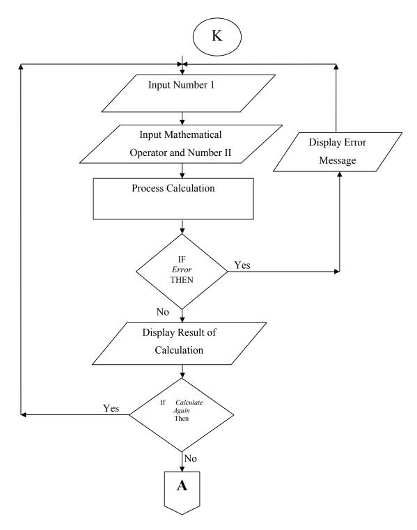
Fig. 13: Program Flowchart for System Calculator
