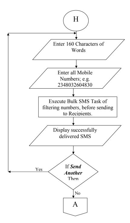
Fig. 10: Program Flowchart for BulkSMS
