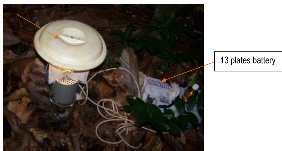
Plate 3: The Pirbright light trap (arrowed) used for insect sampling.
