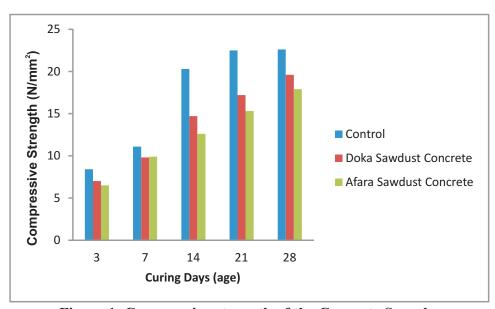
Figure 1. Compressive strength of the Concrete Samples
