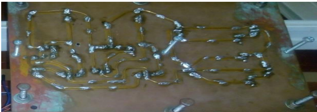
Figure 14: Soldered Surface of the PCB Prototype
