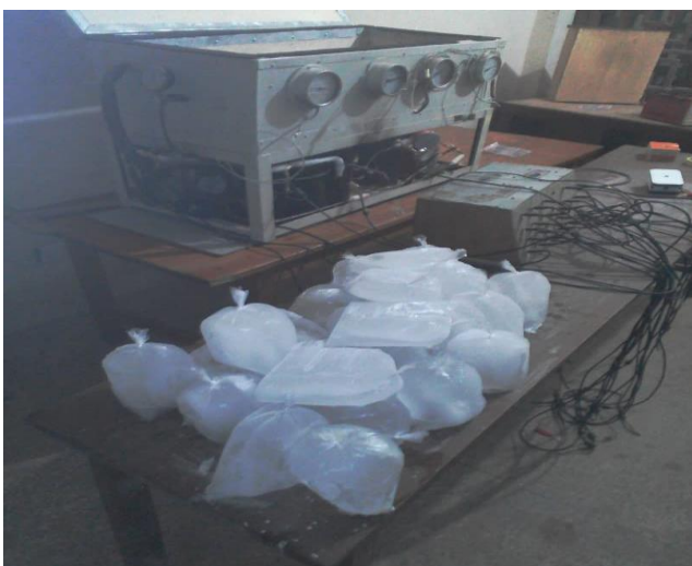
Plate 3: Ice blocks formed within 11 hours of running the main VCR system
