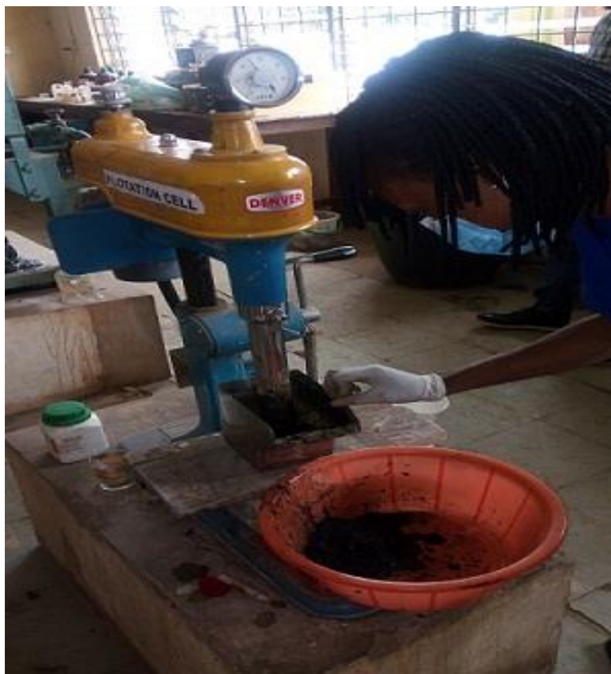
Plate 1: Denver Flotation Cell
