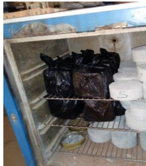
Plate I: MKGPC wrapped and placed in Oven
