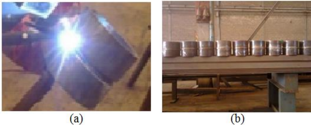
Figure 3: Gas tungsten arc welding process: (a) welding of specimens at 6G position and (b) weld specimens
