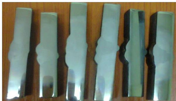
Figure 4: Image acquisition of specimens extracted from the weldments for microhardness profiling
