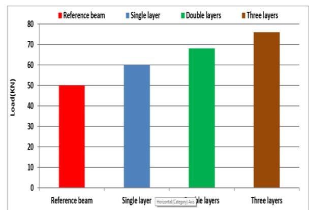
Fig. 7: Ultimate load for control and strengthened beams
