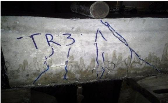
Plate 9: Crack pattern for TL03 beam
