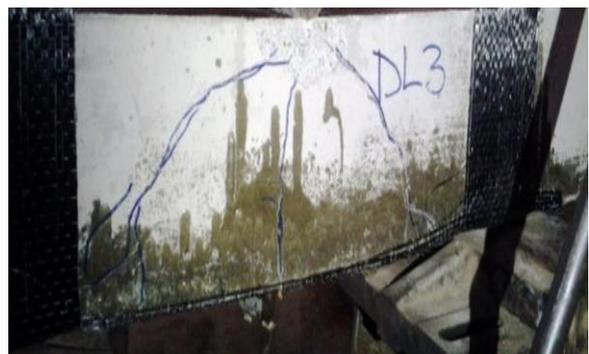
*Plate 7: Crack pattern for DL03 beam*
