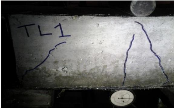
Plate 8: Crack pattern for TL01 beam
