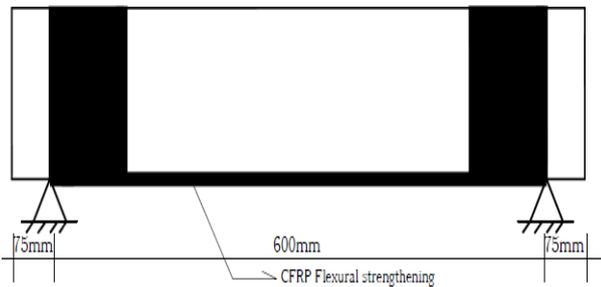
Fig. 2: The strengthening plan of the test beams
