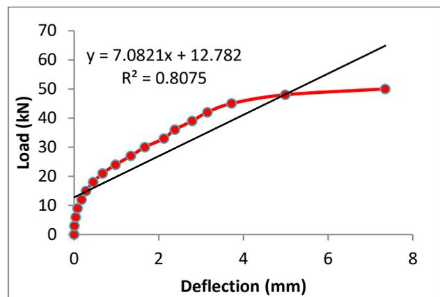
Fig. 3: Average Load deflection plot for the control beams
