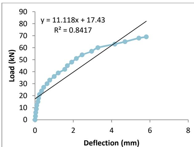
Fig. 5: Average Load deflection plot for double layers beams
