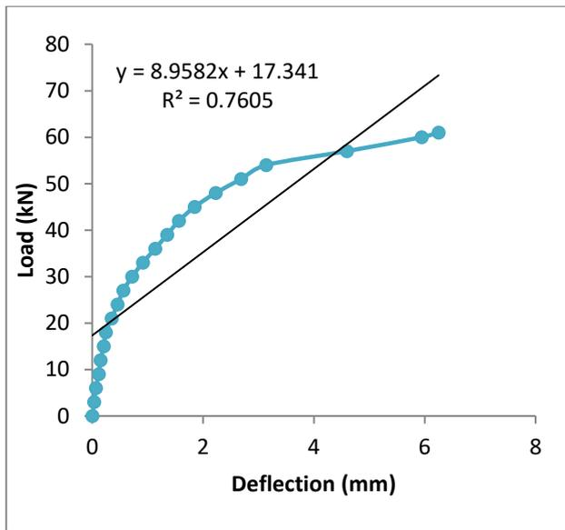
Fig. 4: Average Load deflection plot for single layer beams
