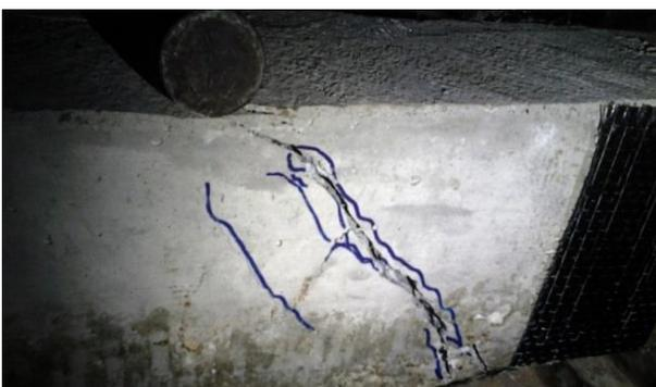
*Plate 4: Crack pattern for SL03 beam*
