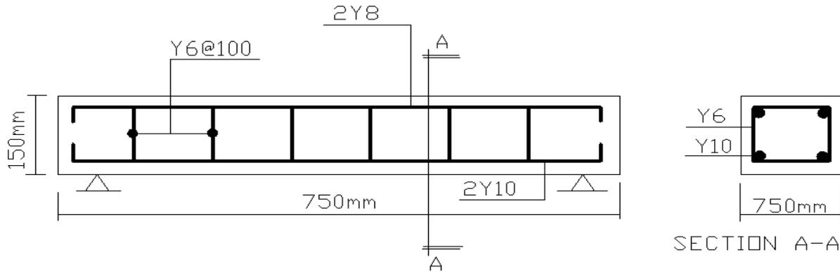
Fig. 1: Structural Detail of the Control Beams
