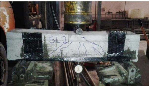
*Plate 3: Crack pattern for SL02 beam*
