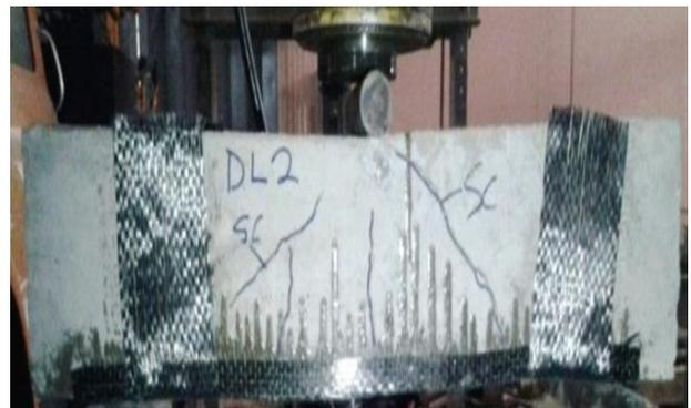
*Plate 6: Crack pattern for DL02 beam*
