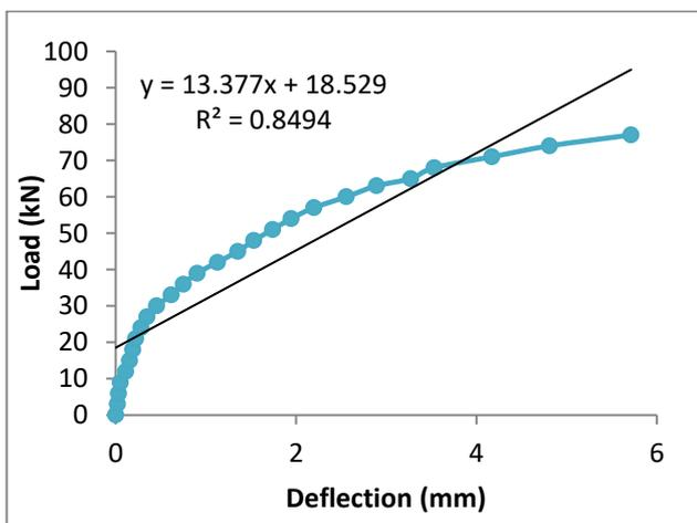
Fig. 6: Average Load deflection plot for three layers beam
