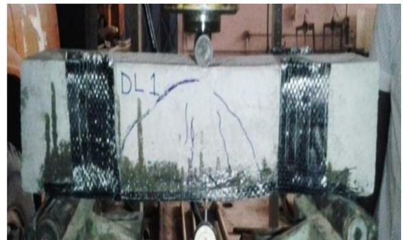
*Plate 5: Crack pattern for DL01 beam*
