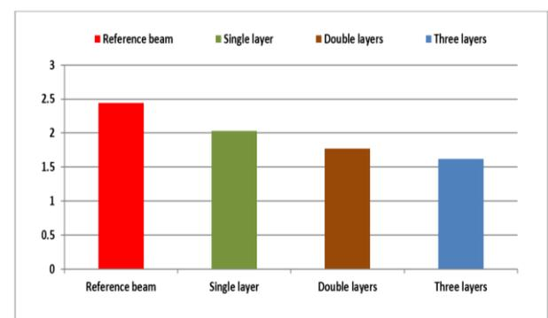
Fig. 8: Ductility index for control and strengthened beams
