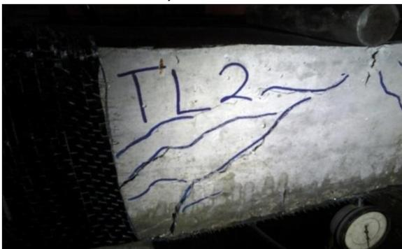
Plate 10: Crack pattern for TL02 beam
