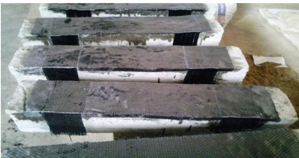
Plate 1: The CFRP Strengthened Beams
