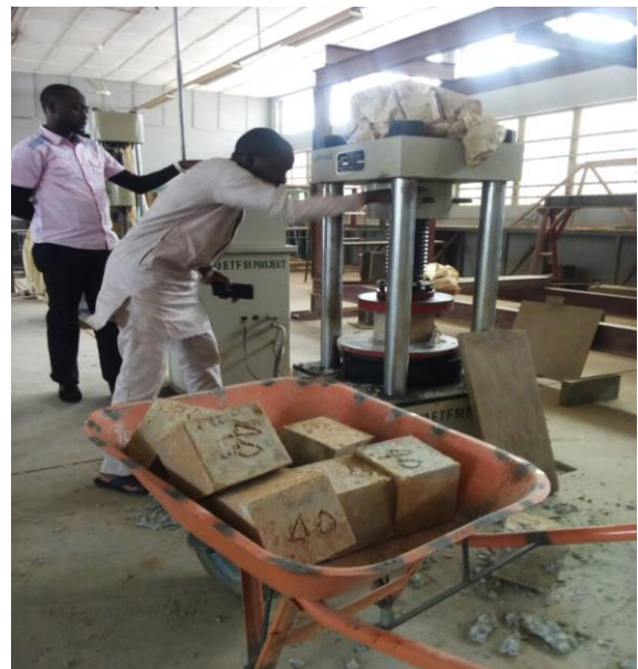
Figure 6: Compressive Strength Tests on Cubes at 28 Days
