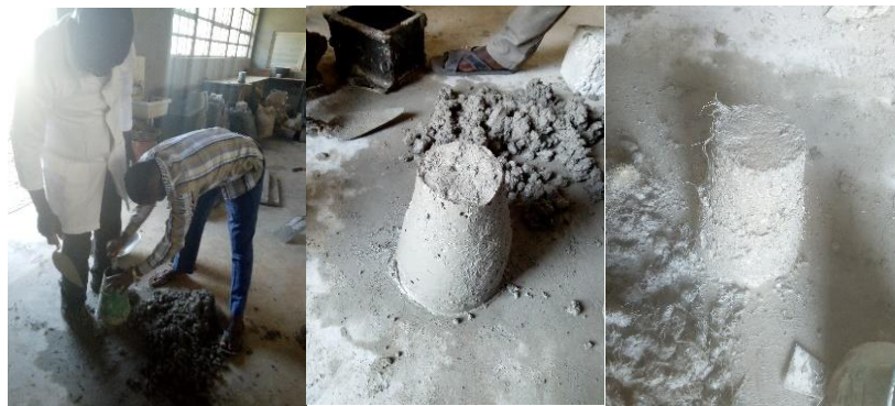
Figure 5: Slump Test to Determine Mix Workability
