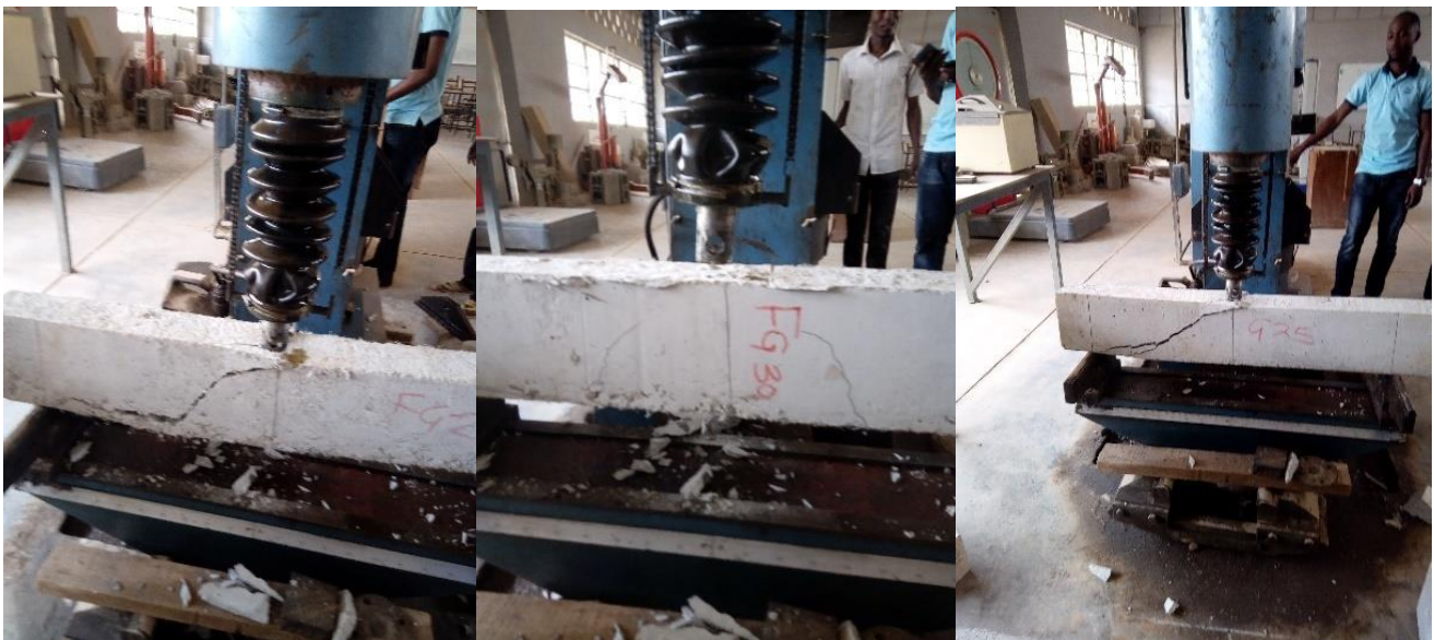
Figure 8: Shear Failures in Beam Test
