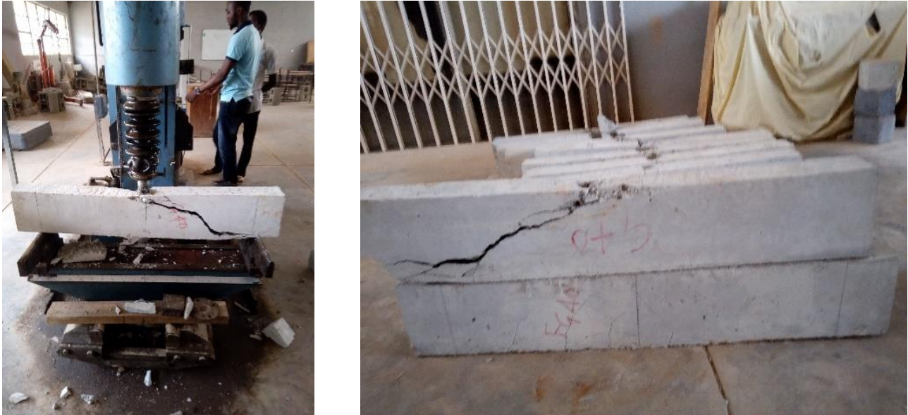
Figure 7: Beam Test Set Up and Tested Beams
