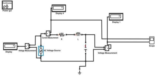
Figure 1: Equivalent circuit model from Simulink (MATLAB)
