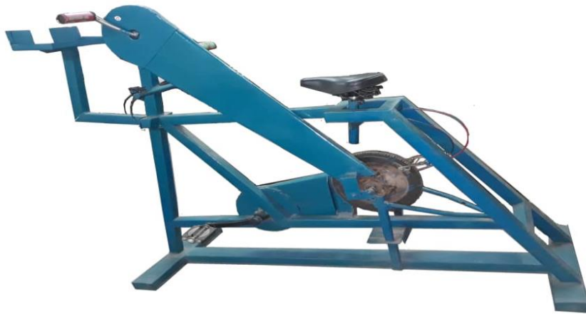
Figure 3: photograph of the side view of bi-modal exercise bike
