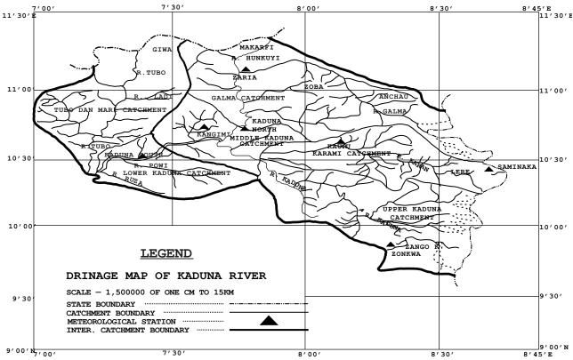
Figure 1: Drainage map of Kaduna River showing rain gauge stations.
