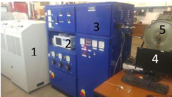
Fig. 4. Experimental Test Rig (1) Programmable power supply (2) Power analyzer (3) Control panel (4) Data acquisition pc (5) induction motor
